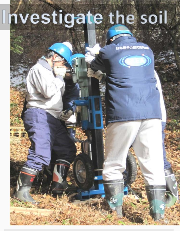
How much radioactive cesium migrates into the soil? How will it change with time? The Headquarters of Fukushima Partnership Operations has been conducting investigations using soil samplers for analyses of cesium depth profile. A soil sampler is a device capable of digging out the soil from the surface in a cylindrical form. This picture shows a soil sampler into the soil in Kawamata Town in Fukushima Prefecture.
